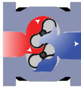
As the impellers continue to turn, the volume of gas in the lower cavity is discharged. Simultaneously, gas is entering the space between the top impeller and housing.
