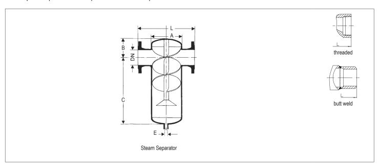
A steam separator (sometimes referred to a moisture separator) is used to separate entrained liquid or moisture droplets that cause "wet steam," a common condition found within most saturated steam systems.
