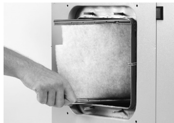
Step 2. Install new inserts in place of the old ones.
